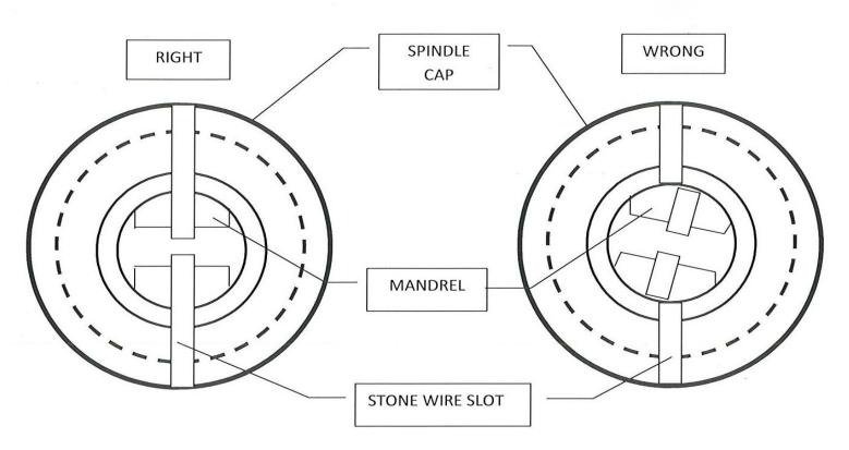
One more additional check – The hardened mandrel pilot bushing in the spindle will, in time, wear and need to be replaced. If these features are right, you will hone more easily and get the results you desire. If you have any questions please give Tennessee Abrasive a call.
